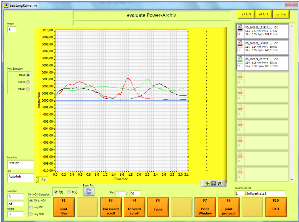
Evaluation window for 3 archived torque recordings of the “Power” function with plot legend.
