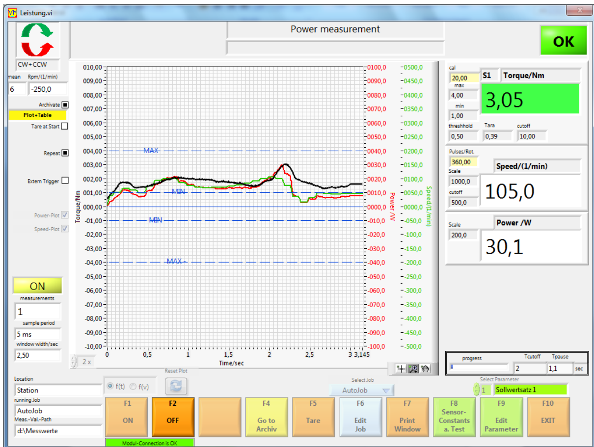
Power function window: Torque, speed and power as a function of time.
