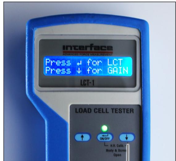
Just push the down arrow key after entering load cell parameters.
