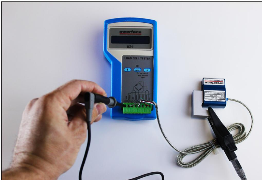
Important: Make sure NOT to connect the SCREEN (shield) and BODY (PINs 7 & 8) at this stage!!
