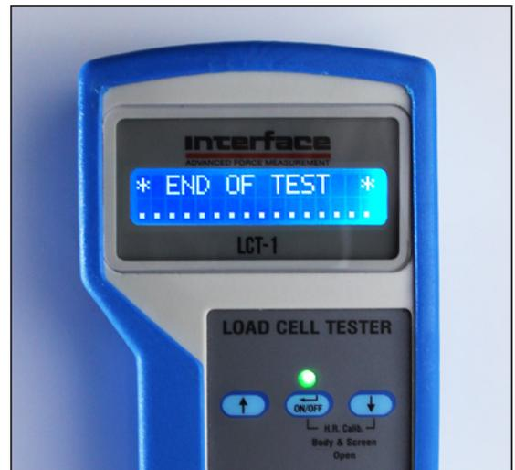
The unit will display "END OF TEST" when complete
