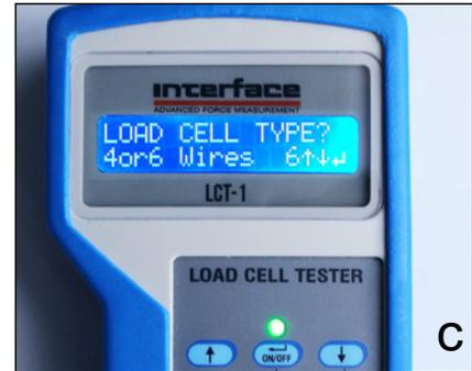
In order to save battery, the backlit LCD display turns off if nothing is done for 15 seconds. To turn the display on, just push any arrow key that won't affect your settings or your current menu. To shut off the unit, press the Enter key (↵) for a few seconds, or leave it on. It will turn off automatically after a few minutes.
