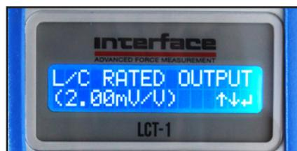
Note: L/C details can be found on the Calibration Certificate that came with the load cell.
