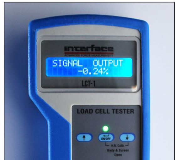
Note: When Load Cell is not loaded, the output should be around 0% (zero balance). Reference the loadcell specification for acceptable zero balance range.
