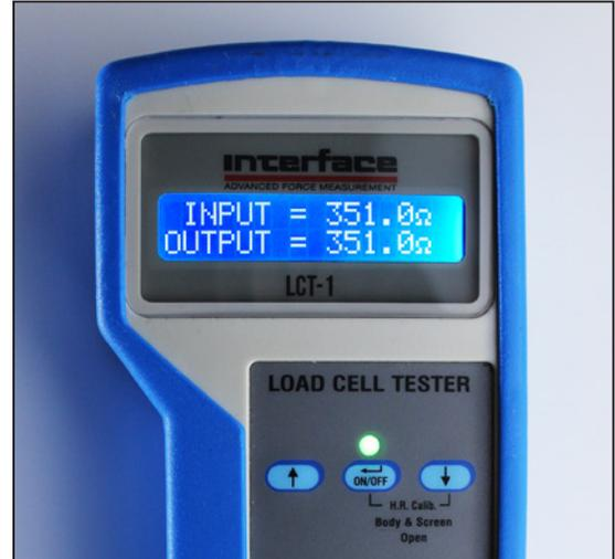
In case of a suspicious reading, the LED turns red.
